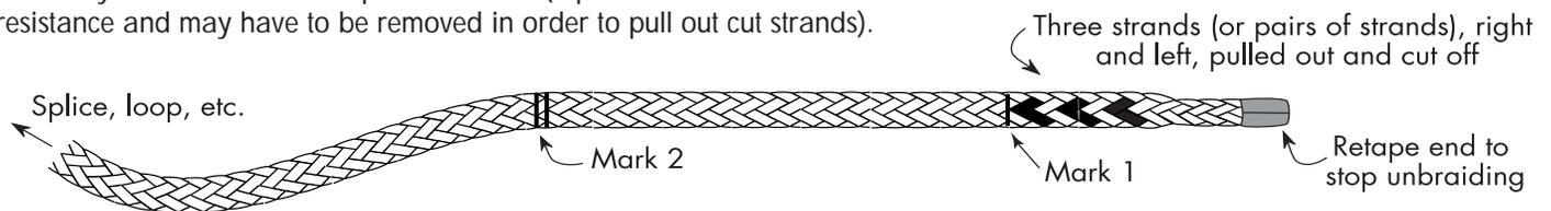
Tapered end will now have only 6 strands remaining. Tape tapered tail tightly to keep from unbraiding.
