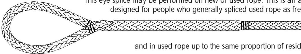
This eye splice may be performed on new or used rope. This is an all-purpose splice technique designed for people who generally spliced used rope as frequently as new rope. By following the procedure below, the splice can retain from 90% to 100% of average new rope strength and in used rope up to the same proportion of residual used rope strength.
